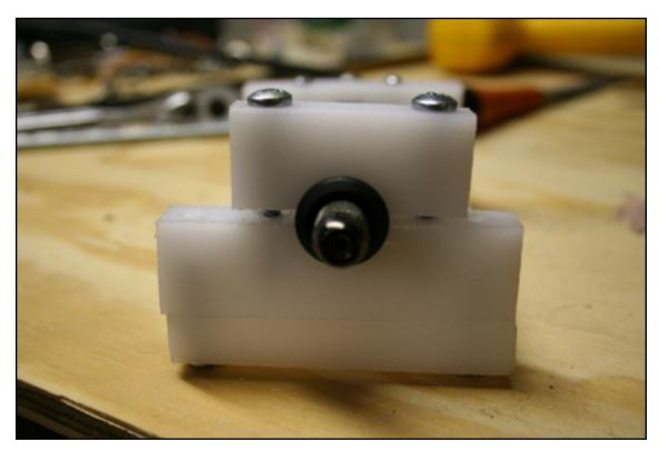
We used a couple of tricks to achieve a nice fit. The strips were cut first, then screwed together with some space to spare. Then we drilled the plastic with a starter hole and used the dremel tool to taper and round out the holes until the fit was perfect.
