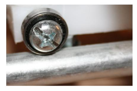
We built this linear slide from a 1/2-inch steel rod and multiple bearing surfaces. It works, but we don't recommend building it if you value your sanity.
