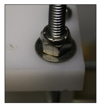
To effectively deal with the minimum space, we had to get tricky. There just isn't enough room in the carrier to mount bearings for the Z axis. Instead, we pressed bushings into the plastic with our vise. Then we added a washer and a lock nut to the threaded rod at the top and bottom of the carrier. Careful tweaking with a pair of wrenches made for very little play. Just how long this setup will stay tight is in question so we'll have to keep an eye on it as we break in the machine.
