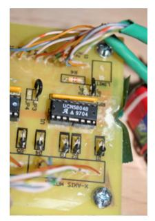
Once you've bought or salvaged a set of motors, you'll need a controller. The controller provides the interface to the computer, drives the motors and can provide some simple feedback to the computer. The stepper controller has to be powerful enough to drive the motors you've selected. We sifted through lots of stepper controller designs looking for one that presented the best value.
