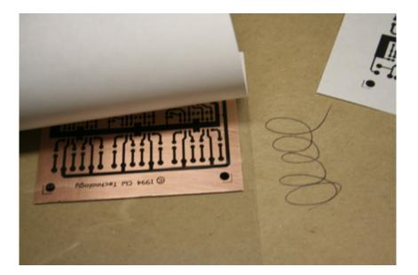
We made our own board using the template from the web page. We used similar techniques to the one in part 4 of our <u>iPod Superdock How-To</u>. We reversed the pdf image using Gimp, and printed it onto a laserprinter transparency. This method doesn't create as nice of a trace as the paper, but it's speedier. Clean the board, and keep the paper backing between the plastic and the iron. Once the toner is ironed, just cool it with water and peel.
