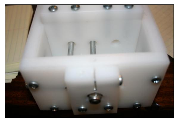
The holes for the rods and screw were drilled at one time on the drill press before assembly. The bearing block was added once the screw was aligned. The locknut isn't necessary. If you want to hand align the machine, This is a good place to add a knob or wheel to spin.
