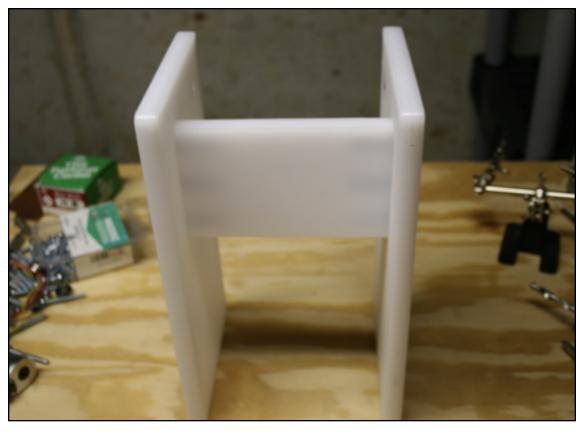
A simple tower constructed of three pieces forms the basis for the rest of the machine. The tower will be mounted to the outer edges of the base. This allows greater side to side movement to maximize the usable area on the table. The center piece of from the same cut as the bottom of the base. To drill the two sides evenly, we screwed them together and drill the mounting holes with the drill press. One the first screw was in, we drilled the rest one at a time.
