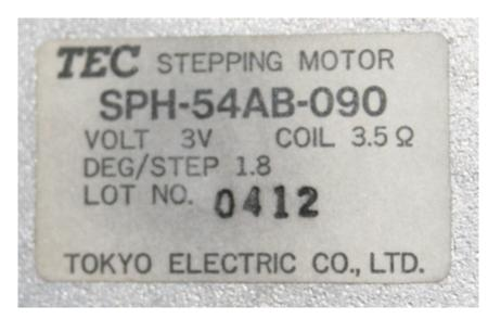
Most stepper motors are labeled. The major points of interest include the voltage, resistance and the number of degrees per step. Knowing the number of degrees per step is vital for configuring the software to properly control the machine later on. For a three axis machine, at the very least you'll want the X and Y axis to both have identical motors. It's not the end of the world if they don't match, but it's more of a pain later on.
