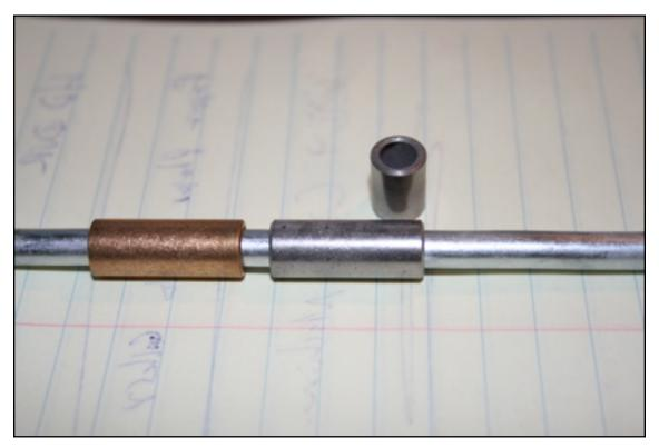
Linear slides are key to the design of a functional machine. These slides are a half successful experiment. We used 1/4-inch steel rod from the hardware store and some brass and steel bushings. The brass material slides easier, but ultimately we think the smaller size and unfinished rod is too prone to binding. Alignment is critical, but they can work well for very short travel.
