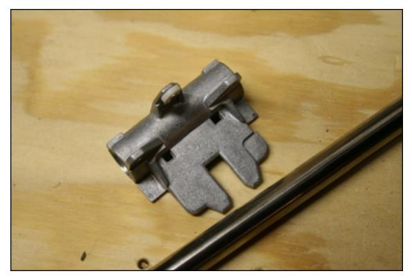
This slide and carrier were salvaged from an old Okidata printer. We decided to use it to smooth out the action for the Y axis.
