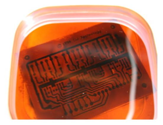
We etched the board using Ferric Chloride from RadioShack in a disposable Zip-Lock container. It needs to be warm and agitated to work well. The acid and hydrogen peroxide solution etches way faster.
