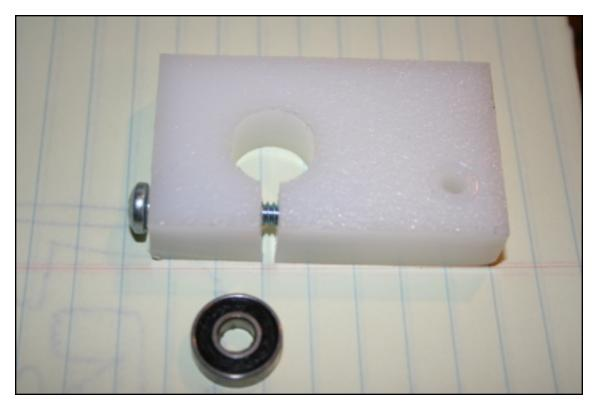
The threaded rod needs to spin freely with the motor, but still needs to be anchored. We picked up a 1/4-inch inner diameter ball bearings off of ebay. We drilled a hole the same size as the bearing, then cut a slot in the piece with a miter saw. Finally, we drilled a hole for a machine screw.
