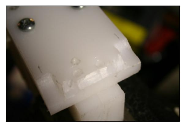
We whipped out the drum sander attachment on our dremel tool and contoured the plastic on the bottom so we could mount the printer slide without compromising the integrity of the cast metal.
